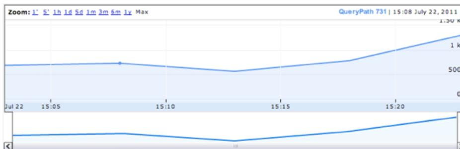
This chart took the information we generated, simplified and reduced to a “per second” interval and develops a timeline trend for the given RPC. This is a simple example, but when implemented with all RPC’s you want to track, you can build a diagram more like:
