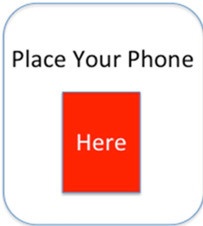
The placard is printed with invisible capacitive ink in a specific pattern that's detected by the touchscreen as multiple simultaneous finger presses. The arrangement of this pattern is used to link Sally's phone with the Local Diner website. The website triggers a second set of messages to the Diameter Routing Agent that first verifies that the phone is actually Sally's, then confirms the charge to the carrier's billing system:
