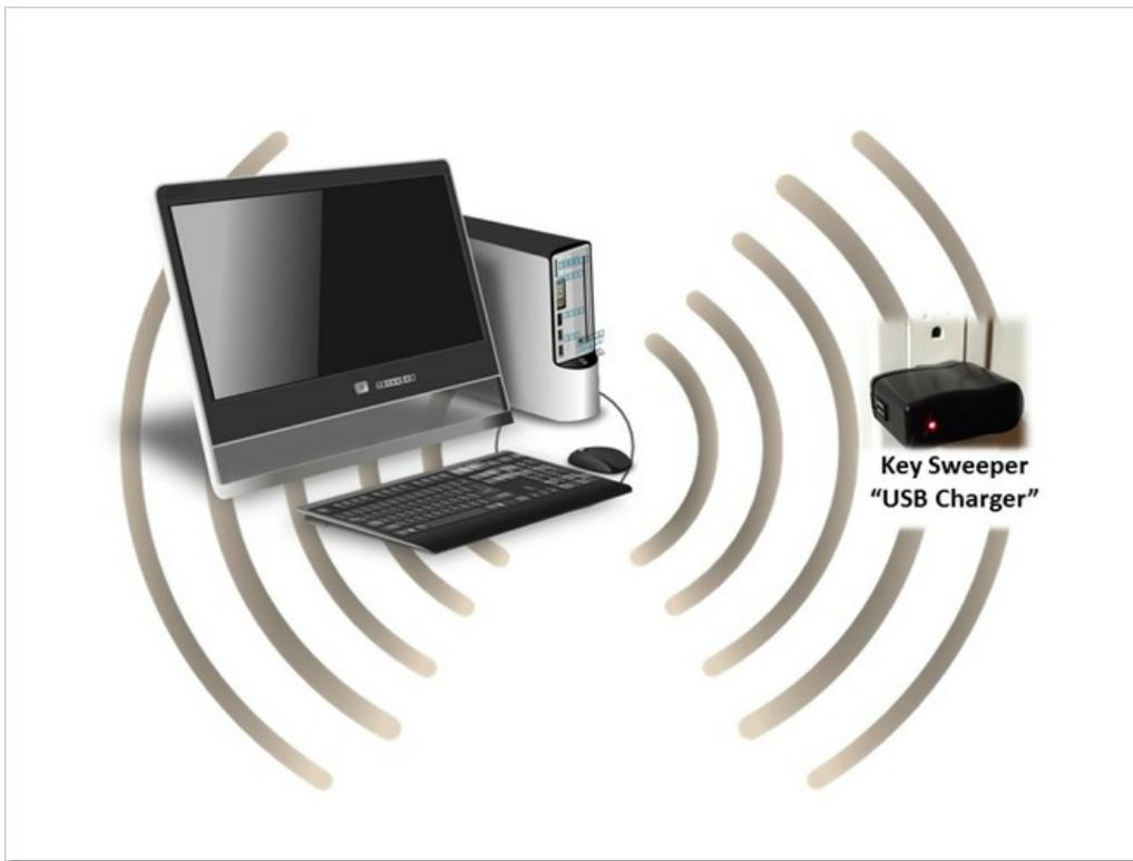
The power of the transmission signal on most wireless keyboards is about 30 feet. So, as long as the KeySweeper is in that range, it should work as advertised. While this particular device works against Microsoft keyboards, rest assured that other devices could be built to work against other keyboard manufacturers as well (Logitech, etc).
