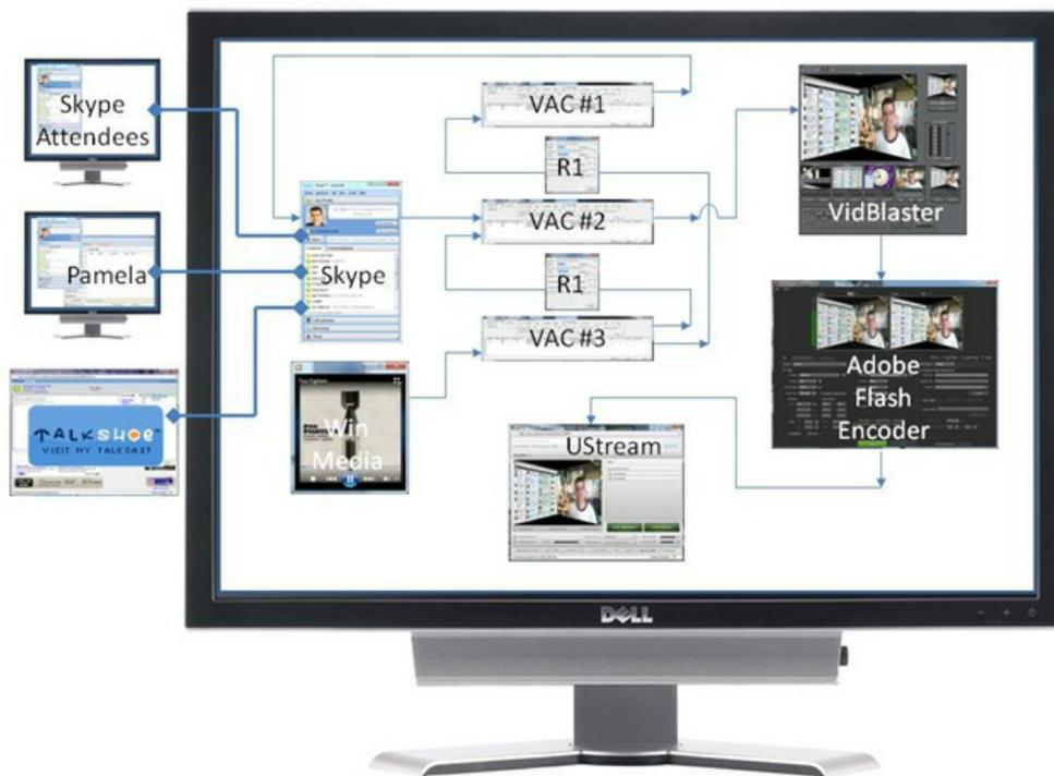
I experimented with a mixing board but ended up with a software only solution that anyone can implement. Everything besides the top left three items in the image were added to enable us to record our Skype podcast as well as stream it to UStream and allow callers with TalkShoe.
